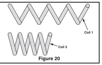
Consider the affect of adding more turns to coiled pipe. The amount of material to push (mass) is increased and the amount of linkage is increased due to more magnets available. This causes the "apparent mass" to increase at a greater rate than would be expected. When making an inductor, the actual inductance is directly proportional to the square of the number of turns.
