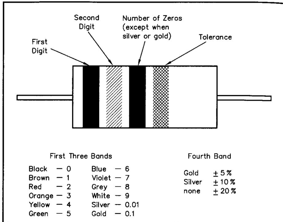
Figure 6-23 — Small resistors are labeled with a color code to show their value. For example, proceeding from left to right, a resistor with color bands of yellow/violet/brown/gold is a 470-Ω resistor with a 5% tolerance.
